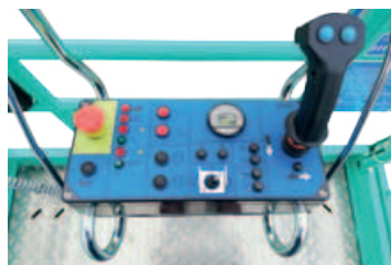
Simple and intuitive control box that can be removed from the basket for loading / unloading the machine
