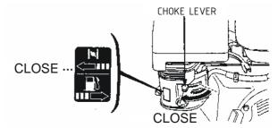
NOTE: Do not use choke lever if the engine is warm or the air temperature is high.
