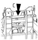
The bucket and platform accessories can be removed by hand by two persons.
