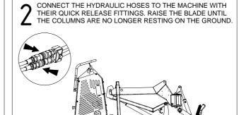
REMOVE THE PINS LOCKING THE COLUMNS AND SLIDE THEM UP UNTIL THEY CAN BE LOCKED INTO THE RAISED POSITION. USE LEVER "F" (REF. 2.1) TO RAISE THE BLADE UNTIL IT IS RESTING ON THE TOOL MOUNT.
