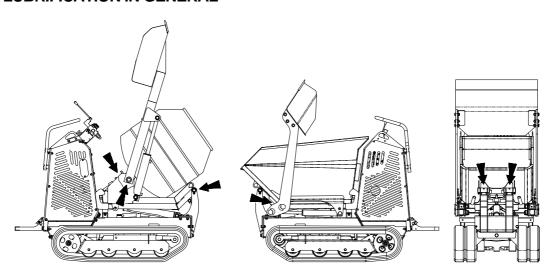
Lubricating the indicated parts when necessary as mentioned in "TABLE OF RECOMMENDED LUBRIFICATION".
