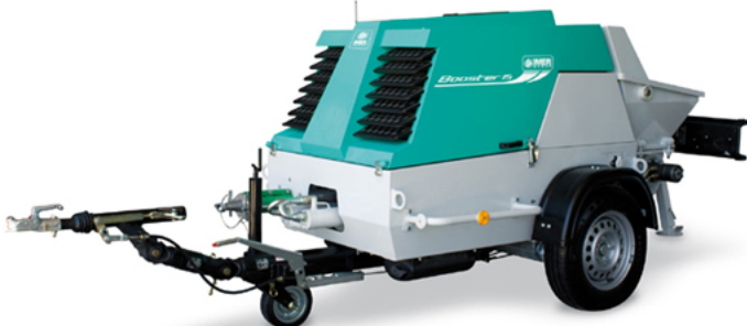
Booster 15, compact yet very powerful, move 20 cubic yards of concrete per hour.
