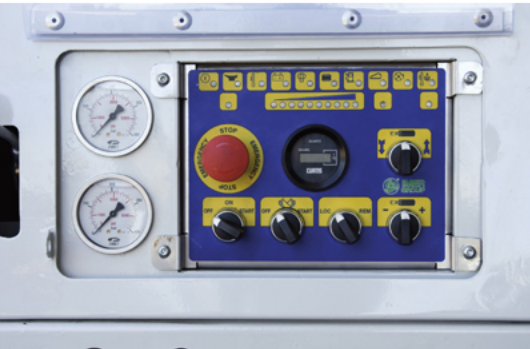
Vibration Isolated Control Panel
