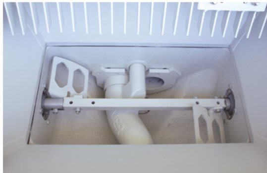
"S" style transfer valve with hydraulic feeder
