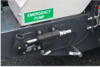
Standard emergency hand pump with ease of access and operation.
