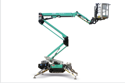
Outstanding accessibility with a 355° rotation (non-continuous) and 124° jib rotation
