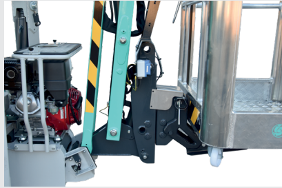
Compact jib assembly hosting both the load sensor and basket rotation system.
