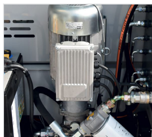
A/C electric power unit
