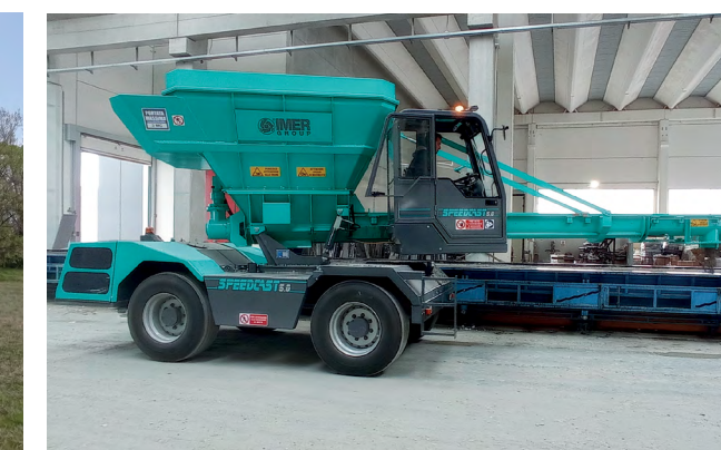
SPEEDCAST makes filling horizontal precast formwork easy with SCC
