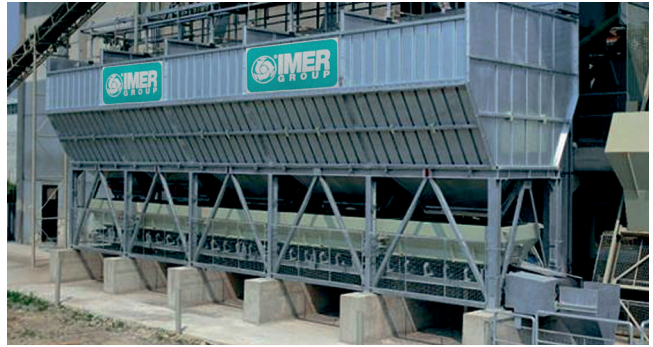
Aggregates storage unit ORU ROME CZ
