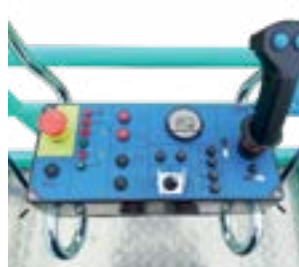
Simple and intuitive control box that can be removed from the basket for loading / unloading the machine
