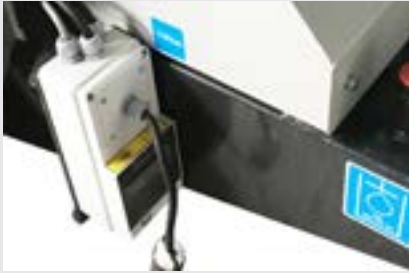
Thermal-magnetic switch panel and power line inlet.
