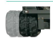
ADJUSTABLE TRACKS Hydraulically adjust the track width for added stability and traction, and to fit through narrow doorwatys and gates for interior or exterior projects
