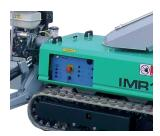
EASY ACCESS In additon to the removeable control box in the basket, the IM R Series includes an easy to access ground control panel.
