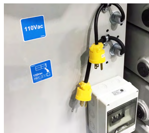
Plug unit for battery charger and power supply on basket with battery level indicator (E and DE versions)
